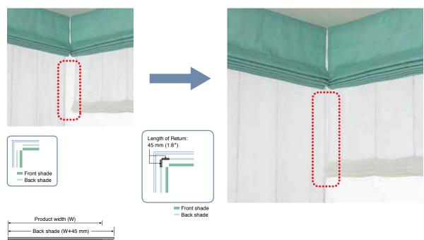
Corner Return is impossible to attach on the operating side. Weight Bar length is the front or back Shade width.
