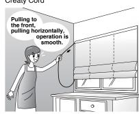
Creaty Cord's heart cam stopper makes it possible to pull the cord at any angle for stop and release operation.
