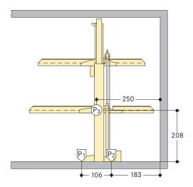
The system units are locked onto the construction frame points of support using heavyduty dowels (having a drilling depth of 10 to 12 cm).
