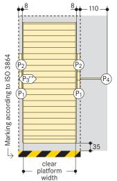
The system units are locked onto the construction frame points of support using heavyduty dowels (having a drilling depth of 10 to 12 cm).
