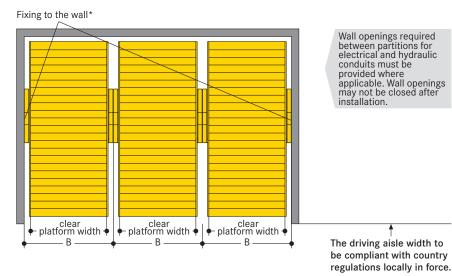
Fixing to the wall on one side (either left or right), is sufficient. The wall shall then be subject to both compressive and traction forces (see statics and construction requirements). With a two-sided fixing system, the wall shall only be subject to compressive forces.
