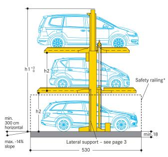
\* Rear and lateral site safety railing, compliant to the DIN EN ISO 13857 standard requirements, is to be supplied by the customer. The height of the safety railing is dependent on the distance from the moving parts.
