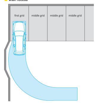
According to GaVo for Baden-Württemberg (07.07.1997/26.01.2011): For parking places with a 90° arrangement at the end of the driving aisle, the entrance width must be min. 275 cm.
