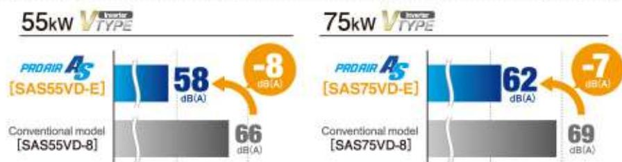
\* Noise values are converted to values for anechoic chamber conditions during full-load operation, at a point 1.5 m in front of the machine (control side) and a height of 1.0 m. The noise value when the machine is actually installed will vary largely depending on the installation environment (effects of surrounding reverberation, etc.). Noise values are also different during airflow control operation.
